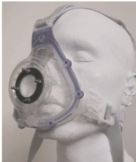
Fig. 1. The collection mask. The sampling masks used to collect exhaled aerosols are shown. Masks were constructed from parts obtained from disposable continuous positive airway pressure masks with the front elbow removed and a disk of electret held in that location with a washer and four bolts, as shown. The mask is shown as it was worn mounted on a dummy head.
