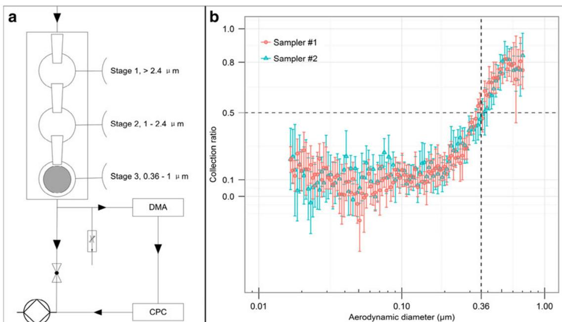
**Fig. 1** a Experimental set up to test the collection efficiency of the RDIs' last impactation stage. b Collection efficiency curves of both RDIs' last impactation stage using QFF as impactation substrate
